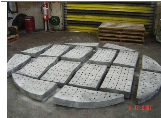
New Zealand's Old warped metal catalyst support – this was an unreliable design
