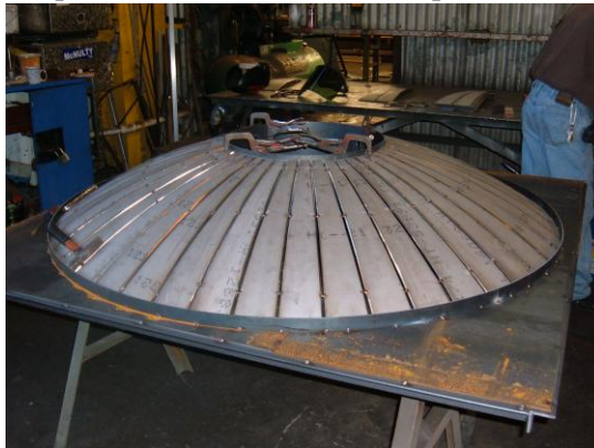
Shop Fabrication of Shroud Lampshade
